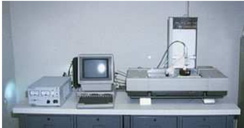
Abbildung 4: 3D-Drucker von Chuck Hull [Quelle: (PC / 3D Printing: What You Need to Know)]
